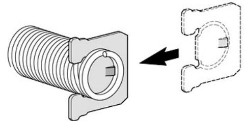
Hammer the metal holder plate (3) into the bottom group.
